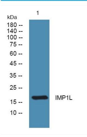
Western Blot analysis of various cells using IMP1L Monoclonal Antibody
