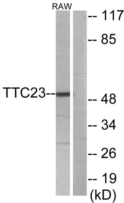
Western blot analysis of lysates from RAW264.7 cells, using TTC23 Antibody. The lane on the right is blocked with the synthesized peptide.
